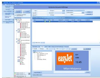
VISTA includes supervision features that check connection status and verify accuracy of images and data displayed on all the display terminals in the airport.
